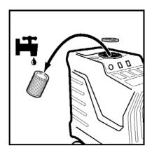
12. When using dry filter, gently remove and wash with water after every use. Allow to dry before re-using.
